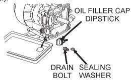
Figure 25. Engine Oil (Draining)
